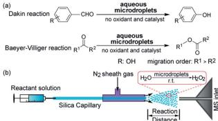
Fig. 1 (a) Dakin oxidation in microdroplets of hydroxybenzaldehydes to phenols and BV oxidation of ketones to esters ( $R^1$  and  $R^2$  denote the migrating groups). (b) Schematic of the experimental setup used to run and monitor the Dakin and BV reactions in aqueous microdroplets sprayed in air.
