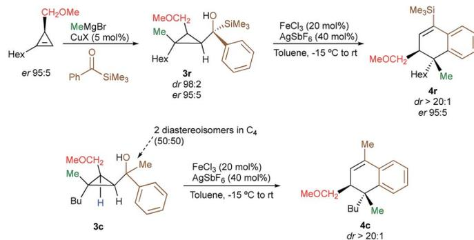
Scheme 3 Diastereo- and enantioselective preparation of dihydronaphthalene.
