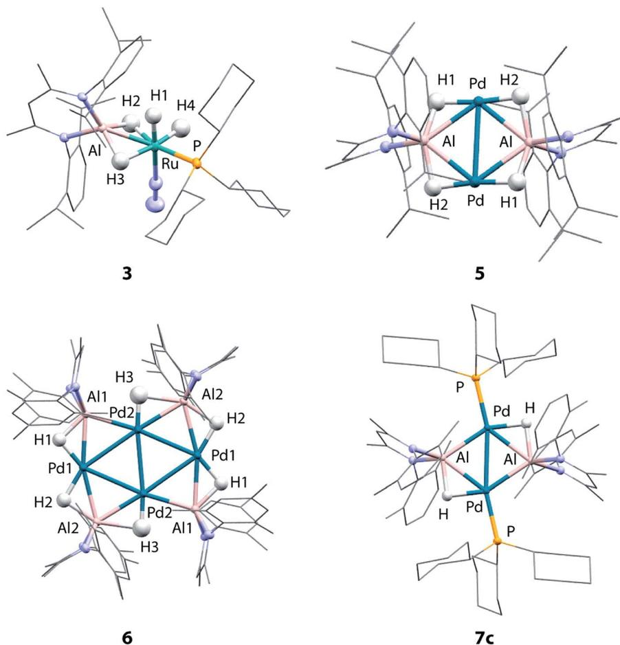
Fig. 2 Crystal structures of **3**, **5**, **6** and **7c**.
