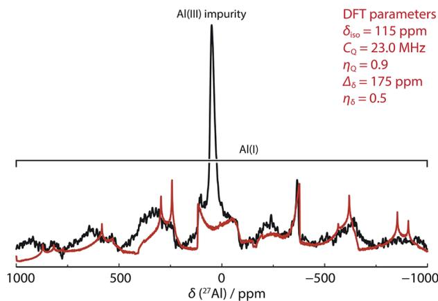
Fig. 3 SS <sup>27</sup>Al MAS NMR spectrum of **8** (black line, 52 464 scans with 1 s relaxation delay) overlaid with simulated lineshape of just the central transition from DFT parameters (red line).
