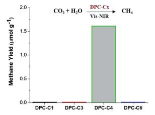
Fig. 11 Photocatalytic  $CO_2$  conversion to methane using DPC-C1, DPC-C3, DPC-C4, and DPC-C6 as catalysts under light (400 to 1100 nm). No conversion in the dark or in the absence of  $CO_2$ . Micro-GC with TCD sensitivity >10 ppm. Error in methane yield for DPC-C4:  $\pm 0.51$ .
