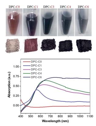
**Fig. 3** (Top) The color of DPC-Cx dispersed in water and powder, and (bottom) absorption spectrum of DPC-Cx with various numbers of growth cycles.
