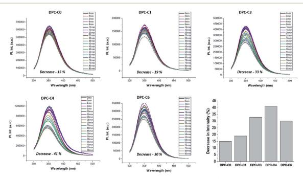
Fig. 12 Steady-state fluorescence of 3.5 mL BSA solution (10  $\mu$ M prepared in PBS buffer of 0.1 mM) in the presence of DPC-C0, DPC-C1, DPC-C3 and DPC-C6 in light (400 to 1100 nm). Excited at 280 nm and emission recorded from 300–500 nm.
