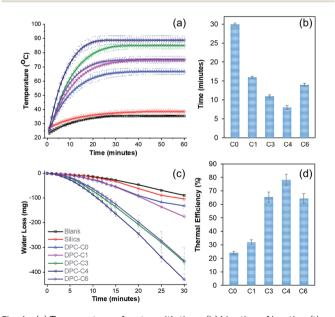
Fig. 4 (a) Temperature of water with time, (b) kinetics of heating (time required to reach 65  $^{\circ}$ C), (c) steam generation (loss of water) over time, and (d) thermal efficiency of steam generation by plasmonic DPC-Cx, using visible to NIR light (400 to 1100 nm wavelength).
