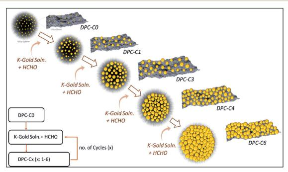
Fig. 1 Cycle-by-cycle growth approach for dendritic plasmonic colloidosomes with varying Au particle sizes and interparticle distances.
