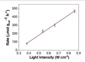
$\begin{tabular}{ll} Fig. 10 & Intensity-dependent photocatalytic rate of COL to CAL using DPC-C4. \end{tabular}$
