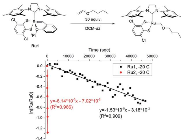
Fig. 3 The plot of  $\ln([Ru]/[Ru]_0)$  vs. time to measure the initiation rates of **Ru1**–**2**<sup>46</sup> at  $-20^\circ\text{C}$  by monitoring the disappearance of the benzylidene signal using <sup>1</sup>H NMR.
