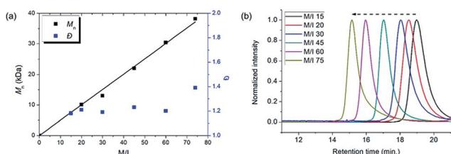
Fig. 1 (a) Plots of the obtained M<sub>n</sub> vs. M/I (solid line shows a fit of the data) and the corresponding D values for P2, and (b) SEC traces of P2 from entries 3–7 in Table 1.
