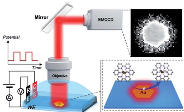
**Scheme 1** Schematic illustration of ECL imaging of electrocatalytic activity on single 2D nanocatalysts. ITO as the working electrode (WE), Ag/AgCl as the reference electrode (RE) and Pt wire as the counter electrode (CE) were used.
