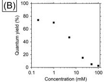
Fig. 2 (A) Absorption (blue) and emission (red) spectra of 0.2 mM TES-ADT in toluene and (B) dependence of TES-ADT concentration in toluene on the QY with excitation at 520 nm.
