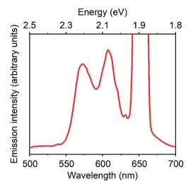
Fig. 3 PUC emission spectrum of a system composed of 1 mM TES-ADT and 20  $\mu$ M PdTPBP, excited at 647 nm.
