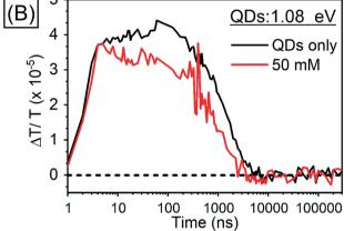
Fig. 6 Kinetics of TA (A) in PbS QDs (1.27 eV) with various concentrations of TES-ADT at 920–930 nm, (B) in PbS QDs (1.08 eV) with 50 mM TFS-ADT at 980–990 nm
