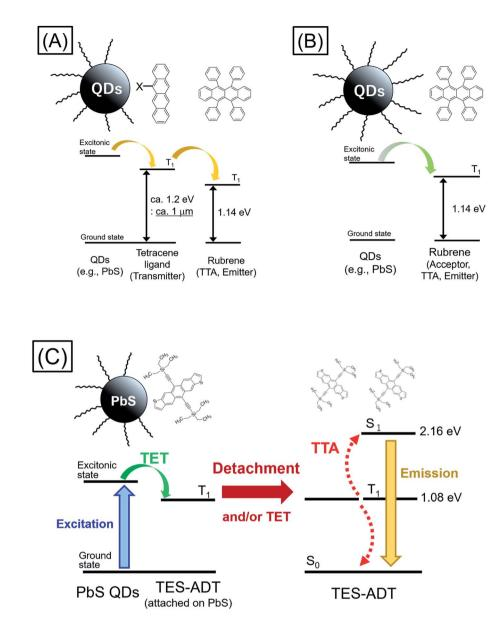
Fig. 1 Schemes of TTA PUC with inorganic semiconductor QDs as the triplet sensitizer; (A) via triplet transmitter ligand (e.g., rubrene and QDs modified with tetracene derivative), (B) direct energy transfer (e.g., rubrene and QDs), (C) this work (TES-ADT/PbS QDs).
