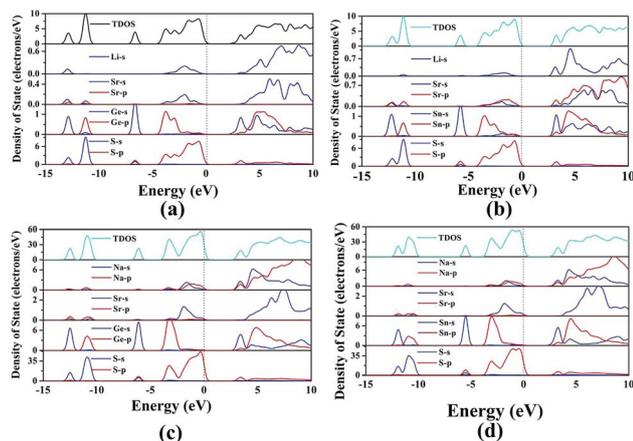
Fig. 5 Total and partial density of states (TDOS and PDOS) of title compounds: (a)  $\text{Li}_2\text{SrGeS}_4$ , (b)  $\text{Li}_2\text{SrSnS}_4$ , (c)  $\text{Na}_2\text{SrGeS}_4$ , and (d)  $\text{Na}_2\text{SrSnS}_4$ .
