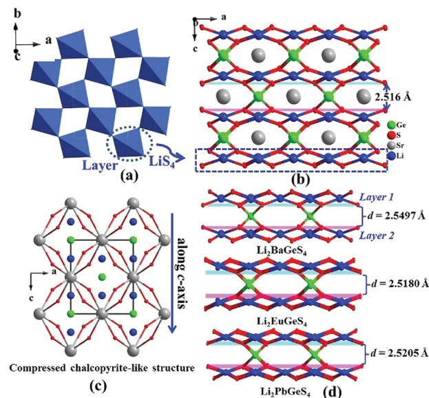
Fig. 1 (a) Corner-sharing  $(\text{LiS}_4)_n$  layer; (b) whole crystal structure of  $\text{Li}_2\text{SrGeS}_4$  (Sr–S bonds omitted for clarity); (c) 3D network structure composed of edge-sharing  $\text{SrS}_8$  dodecahedra (Ge–S and Li–S bonds omitted for clarity); (d) comparison of the interlayer spacing between adjacent  $(\text{LiS}_4)_n$  layers in Li-based materials.
