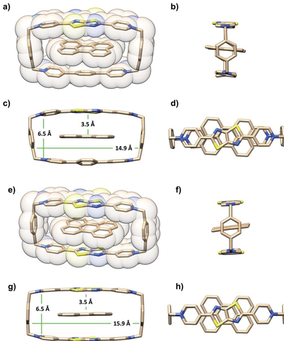
Fig. 2 A blend of tubular and space-filling representations of the solid-state structure of (a–d) Per ⊂ TTzExVBox<sup>4+</sup> and (e–h) Per ⊂ TTzBox<sup>4+</sup> showing the main structural parameters. Counterions and residual solvent molecules are omitted for clarity.
