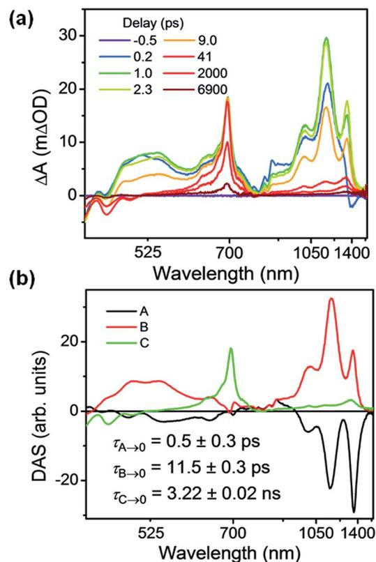
Fig. 4 (a) fsTA spectra and (b) decay-associated spectra (DAS) of Per  $\subset$  TTzExVBox<sup>4+</sup> in CH<sub>3</sub>CN excited at 414 nm (A) formation of Per<sup>2+</sup>-TTz<sup>2+</sup>, (B) decay of Per<sup>2+</sup>-TTz<sup>2+</sup>, (C) decay of unbound <sup>1</sup>\*Per). The wavelength axis is plotted in reciprocal space. Time constants are for the representative data set shown here; averages and standard deviations from multiple experiments are given in Table 1.
