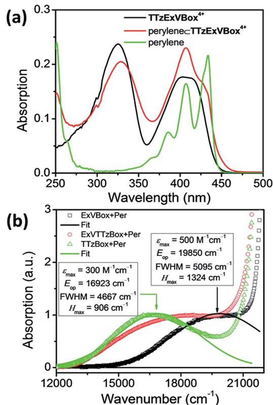
Fig. 3 (a) Steady-state absorption spectra of TTzExVBox<sup>4+</sup>, Per and Per  $\subset$  TTzExVBox<sup>4+</sup> in CH<sub>3</sub>CN. The concentration of Per in the latter two solutions is kept the same. (b) CT bands in Per  $\subset$  ExVBox<sup>4+</sup>, Per  $\subset$  TTzBox<sup>4+</sup>, and Per  $\subset$  TTzExVBox<sup>4+</sup>, and extracted couplings.
