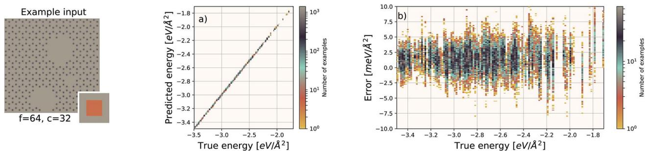
Fig. 7 Left: an example porous graphene sheet. (a) The true (DFT) vs. predicted (EDNN) total energy in  $\text{eV } \text{\AA}^{-2}$ . The tight clustering along the diagonal indicates the EDNN performs well at predicting the total energy. (b) The error (DFT energy – EDNN energy), in  $\text{meV } \text{\AA}^{-2}$ , is very close to zero.
