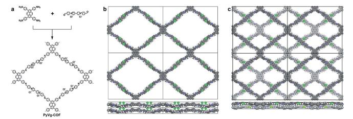
Fig. 1 (a) Schematic representation of the synthesis of the PyVg-COF. (b) Top and side views of the PyVg-COF in the eclipsed AA stacking mode (C: grey; N: blue; Cl: green; H: white). (c) Top and side views of the PyVg-COF in the staggered AB stacking mode (dark grey and light grey show the two staggered layers).
