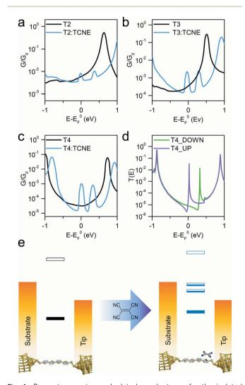
Fig. 4 Room temperature calculated conductance for the isolated molecules (black line) and complexed with TCNE (blue) for compounds T2 (a), T3 (b) and T4 (c), along with a representative spin-polarised *T*(E) curve for the TCNE complex of T4 (d). Schematic diagram (e) showing the position of the DFT resonances for T4 respective to the two electrodes before and after TCNE complexation. The part-filled CT resonances in the HOMO–LUMO gap are responsible for the observed increase in conductance.
