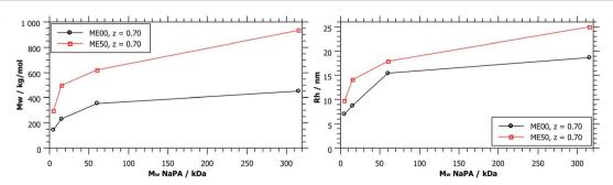
Fig. 6  $M_{\rm w}$  and  $R_{\rm h}$  obtained from static and dynamic light scattering as a function of  $M_{\rm w}$  (NaPA), comparing different droplet sizes for a charge ratio z=0.7.  $M_{\rm w}$  (ME00) = 52 kg mol<sup>-1</sup> and  $M_{\rm w}$  (ME50) = 110 kg mol<sup>-1</sup>.
