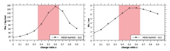
Fig. 3 Apparent  $M_{\rm w}$  and  $R_{\rm h}$  obtained from static and dynamic light scattering show the presence of differently sized aggregates of ME and PE depending on the charge ratio z. Metastable samples (shaded in red) were measured while still being homogeneous, typically being 3-5 days old. Measured values for longer NaPAs are given in Fig. S4.†
