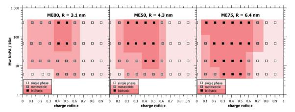
Fig. 1 Phase diagrams showing the biphasic and the metastable regions for ME00 (R = 3.1 nm), ME50 (R = 4.3 nm) and ME75 (R = 6.4 nm) at c (surfactant) = 100 mM, mixed with NaPA of different molecular weights and at different charge ratios z.
