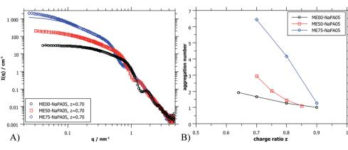
Fig. 5 (A) SANS scattering curves (ME00 and ME50 from PAXY at LLB and ME75 from D11 at ILL) of complexes formed with differently sized microemulsion droplets and NaPA05. Solid lines were calculated for a cylindrical arrangement of the droplets.<sup>45</sup> (B) Aggregation number  $N_{\text{agg}}$  of ME droplets contained in the aggregates as deduced from extrapolated I(0) values of SANS curves (for details see the ESI†).
