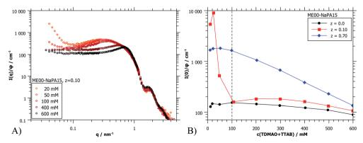
Fig. 8 (A) Selected SANS curves (PAXY at LLB) of the dilution series of ME00–NaPA15 complexes, normalized by volume fraction  $\varphi$ . (B)  $I(0)/\varphi$  for three different charge ratios; the charge ratios were chosen to be below and above the two phase region of the phase diagram. The dotted line shows the concentration of all other samples presented in this work.
