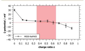
Fig. 2 ζ-Potential of microemulsion-polyelectrolyte complexes at different charge ratios, showing the transition from positively charged microemulsion droplets to negatively charged complexes. The metastable region is shaded in red.
