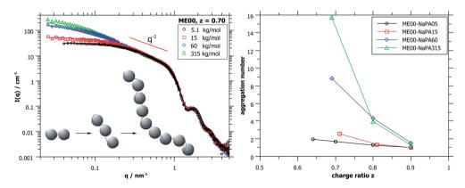
Fig. 7 (A) Comparison of complexes formed with ME00 and NaPA of different  $M_{\rm w}$  at a charge ratio z=0.7 in the polyelectrolyte excess, where the biggest complexes are formed (NaPA05 and 15 from PAXY at LLB and NaPA60 and 315 from V4 at HZB). Solid lines were calculated for a cylindrical arrangement of the droplets. (B) Aggregation number  $N_{\rm agg}$  deduced from extrapolated I(0) values of SANS data, compared for different NaPA chain lengths.
