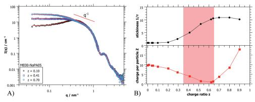
Fig. 4 (A) Fitted SANS spectra (PAXY at LLB) of three ME00–NaPA05 samples, showing the good agreement of the chosen structure factor model with the measured data points (fit curves as solid red lines). (B) Fit parameters 'stickiness'  $1/\tau$  and 'charge per particle' Z obtained from fitting the structure factor in dependence of the charge ratio z. The metastable region is shaded in red.
