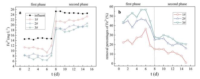
Fig. 6 (a)  $Fe^{2+}$  residual concentration in Columns 1, 2, 3. (b) The removal percentage of  $Fe^{2+}$  in Columns 1, 2, 3. Influent is the  $Fe^{2+}$  concentration in influent water of AMD. 1#, 2# and 3# in (a) are the residual Fe<sup>2+</sup> concentration in AMD after repairing AMD with Column 1, Column 2 and Column 3 respectively. 1#, 2# and 3# in (b) are the removal percentage of Fe<sup>2+</sup> in AMD by the three dynamic columns corresponding to (a) respectively.
