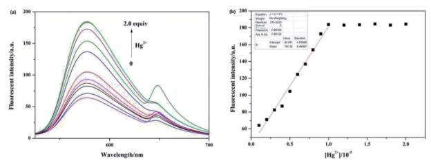
Fig. 5 (a) The fluorescence spectra of sensor Pyr-Rhy (10  $\mu$ M) with the increasing concentration of Hg<sup>2+</sup> ion (0–2.0 equiv.) in ethanol solution; (b) the linear fit between sensor Pyr-Rhy and Hg<sup>2+</sup> ion.
