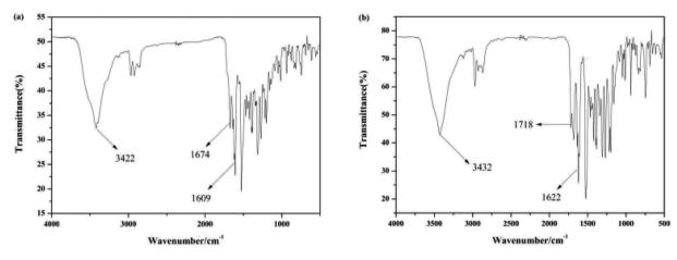
Fig. 10 (a) The FT-IR spectrum of sensor Pyr-Rhy; (b) binding FT-IR spectrum of Pyr-Rhy-Hg<sup>2+</sup>
