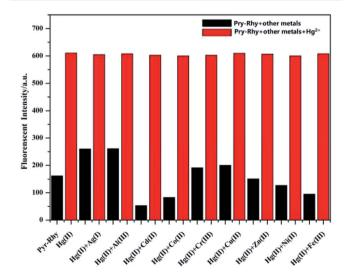
Fig. 7 The black bars represent the fluorescent intensity of sensor Pyr-Rhy and various metal ions (1.0 equiv.) in DMSO/ $H_2O$  (1/1, v/v) solution; the red bars represent the fluorescent intensity of sensor Pyr-Rhy and  $Hg^{2+}$  (1.0 equiv.) in DMSO/ $H_2O$  (1/1, v/v) solution.
