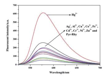
Fig. 3 Fluorescence spectra of sensor Pyr-Rhy (10  $\mu$ M) in the presence of various metal ions (10  $\mu$ M) in DMSO/H<sub>2</sub>O (1/1, v/v) solution ( $\lambda_{ex}$  = 525 nm).
