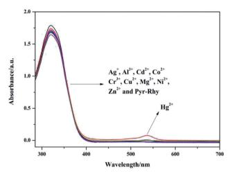
Fig. 2 UV-vis absorption spectra of sensor Pyr-Rhy (10  $\mu$ M) upon addition of different metal ions (10  $\mu$ M) in DMSO/H<sub>2</sub>O (1/1, v/v) solution.
