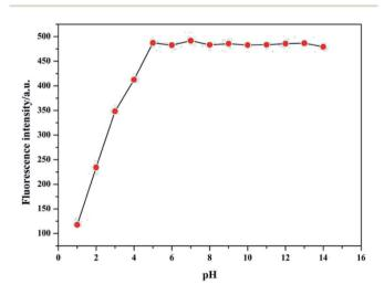
Fig. 6 Effect of pH on the fluorescence intensity of sensor Pyr-Rhy toward  $Hg^{2+}$  in DMSO/ $H_2O$  (1/1, v/v) solution.
