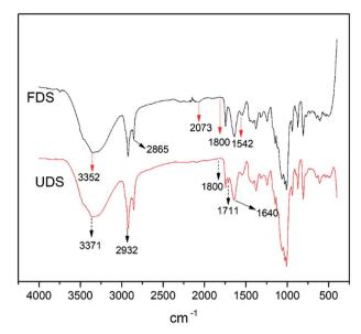
Fig. 11 FTIR spectra of fresh date seed (FDS) and used date seed (UDS).
