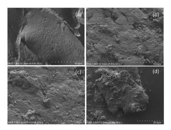
Fig. 9 FESEM images of (a) fresh date seed (10  $\mu$ m), (b) used date seed (10  $\mu$ m), (c) used date seed (5  $\mu$ m), (d) used date seed (20  $\mu$ m).
