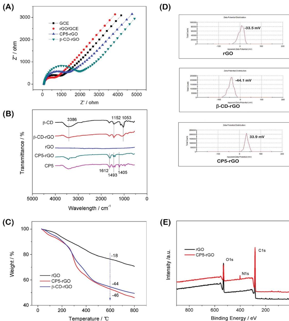
Fig. 3 The EIS characterization of GCE,  $\beta$ -CD-rGO/GCE and CP5-rGO/GCE via  $[\text{Fe}(\text{CN})_6]^{3-/4-}$  (2.0 mM) redox couple (1 : 1) with KCl (0.1 M) as supporting electrolyte (A). FTIR spectra of  $\beta$ -CD,  $\beta$ -CD-rGO, rGO, CP5-rGO and CP5 (B). TGA curves of rGO, CP5-rGO and  $\beta$ -CD-rGO (C). Zeta potentials of rGO,  $\beta$ -CD-rGO and CP5-rGO (D). XPS survey spectra of rGO and CP5-rGO (E).
