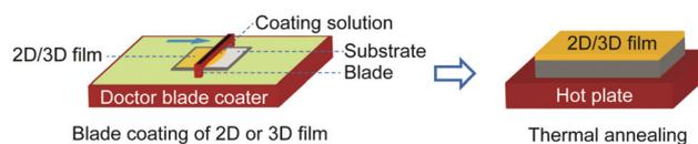
Fig. 1 Schematic illustration of the doctor-blade setup used for the deposition of the 2D PEA<sub>2</sub>PbI<sub>4</sub> and reference 3D FAPbI<sub>3</sub> perovskite films.
