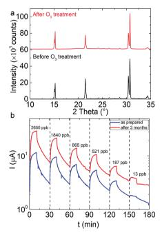
Fig. 5 (a) Corresponding XRD patterns of the sensing material before (lower) and three months after the ozone exposure (upper) (images are presented in Fig S3†). (b) Electrical response of an all-inorganic perovskite nanocube sensor as a function of the ozone exposure time at various concentrations in the as-prepared state (blue curve) and that obtained upon the sensor storage for three months under ambient conditions (red curve).
