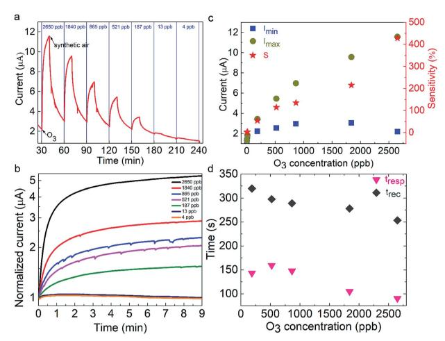
Fig. 2 Electrical response of the all-inorganic perovskite nanocubes as sensing materials upon applying various ozone concentrations from 2650 down to 4 ppb as a function of the ozone exposure time (a and b). Sensitivity (S) and response ( $t_{res}$ ) and recovery time ( $t_{rec}$ ) as a function of gas concentration of the nanocube-based sensor (c and d).
