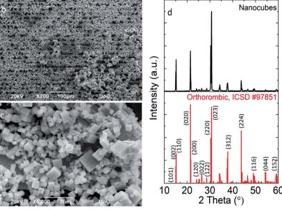
Fig. 1 Schematic representation of the ozone sensor fabrication based on  $CsPbBr_3$  nanocubes (a), SEM images (b and c) and X-ray diffraction pattern ((d) black curve) of the nanocubes prior to ozone treatment. A reference pattern of the orthorhombic (ICSD, #97851) crystal structure of  $CsPbBr_3$  is provided for comparison ((d) red curve).
