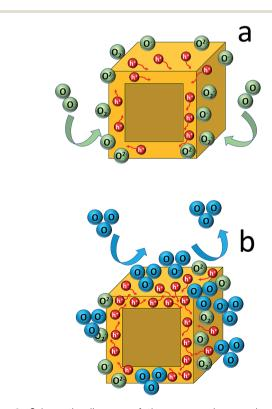
Fig. 6 Schematic diagram of the gas sensing mechanism under ambient conditions (a) and after ozone exposure (b).
