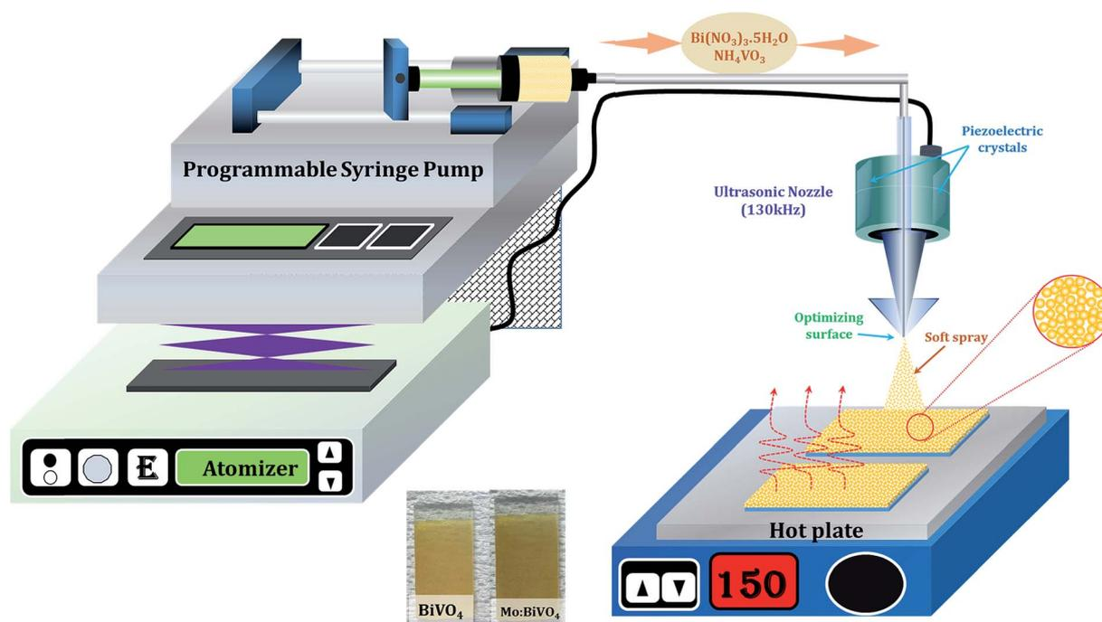
Fig. 1 Schematic of concurrently pumped ultrasonic spray coating for pristine and Mo-doped BiVO<sub>4</sub> thin film deposition.
