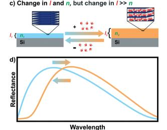
Fig. 2 Stimulus sensing with a photonic thin film. A change caused by a stimulus in the refractive index a), or layer thickness b), or both c), can result in a change of the displayed structural color d). In the case of c), which is the default situation in nanosheet-based thin films, the change in the layer thickness is much more pronounced compared to the decrease of the refractive index. Therefore, an overall redshift in the reflectance spectrum is observed, d).
