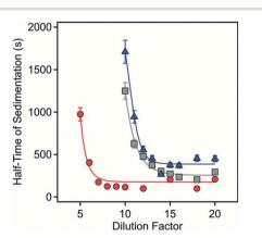
Fig. 6 Half time of sedimentation as a function of the dilution factor for sample 1 (circles), sample 2 (squares) and sample 3 (triangles).
