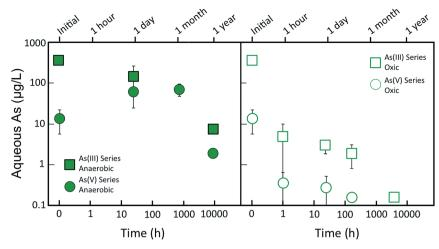
Fig. 1 Aqueous As concentration during aging of green rust suspensions in anoxic (solid symbols) and oxic (open symbols) environments. The circles represent experiments with initial As(v) and the squares represent experiments with initial As(III). Data points and error bars represent the average and standard deviation of replicate aqueous As measurements, with some error bars smaller than the symbol.
