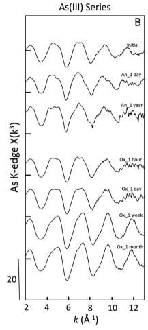
Fig. 6 As K-edge EXAFS spectra of aging samples in As(v) experiments (A) and As(III) experiments (B). Reference spectra of As(v) co-precipitated with magnetite (AsV Co-PPT Mag) and adsorbed to magnetite (AsV Ads Mag) are given for comparison. The \* symbols indicate EXAFS features consistent with As occupying the tetrahedral Fe site in magnetite.
