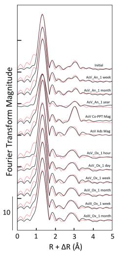
Fig. 7 Fourier-transformed As K-edge EXAFS spectra of select aging samples in As(v) and As(III) experiments. The shell-by-shell fitting output (dotted red lines) is overlain to the data (solid black lines). In addition to aging samples, the fits of As(v) co-precipitated with magnetite (AsV Co-PPT Mag) and adsorbed to magnetite (AsV Ads Mag) are given.
