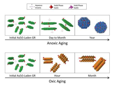
Fig. 8 Models of the transformation of As(v)-laden green rust (GR) over time in anoxic (top panels) and oxic conditions (bottom panels). The initial GR transforms into magnetite (blue spherical crystals) in a year in the anoxic system, whereas lepidocrocite (brown layered crystals) forms in an hour in the oxic system. Experiments with As(III)-laden GR followed similar trends.
