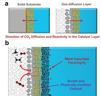
Fig. 5 (a) Schematic of the directional change in CO<sub>2</sub> transport for fullyaqueous and gas-diffusion layer CO2 reduction catalysts. (b) Potential advantages of a change in the CO2 transport and reaction direction inside a catalyst layer. A buried catalyst layer may be inherently more stable and protected from both contaminants and restructuring while still having access to CO<sub>2</sub>.
