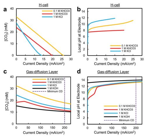
Fig. 3 Simplified predictions of the electrode concentration of  $CO_2$  and pH for commonly-used electrolytes as a function of current density in an (a and b) H-cell with a 50  $\mu$ m  $CO_2$  diffusion thickness and, (c and d) a gas-diffusion layer with a 50 nm  $CO_2$  diffusion thickness and liquid diffusion layer of 200  $\mu$ m. A Faradaic efficiency of  $CO_2$ -to-CO of 90% is assumed.
