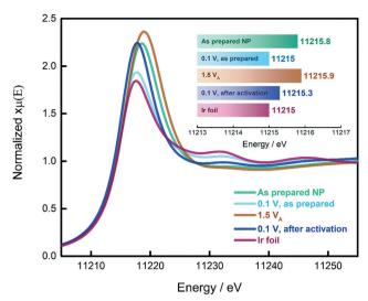
Fig. 3 Normalized Ir L3-edge XANES spectra of the Ir NP recorded at different potentials under steady state conditions. V<sub>A</sub> stands for "anodic". The inset shows the energy at the maximum of the first derivative of the XANES spectra for the different samples. The density of the data points in the plots is 5 points per eV.
