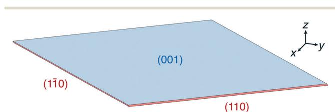
**Fig. 7** Steady state crystal shape obtained from simulation at  $C = 1.2 \text{ nm}^{-3}$ . The blue colored large surface corresponds to face  $\{00\bar{1}\}$  and the red colored thin surfaces correspond to face  $\{1\bar{1}0\}$ .
