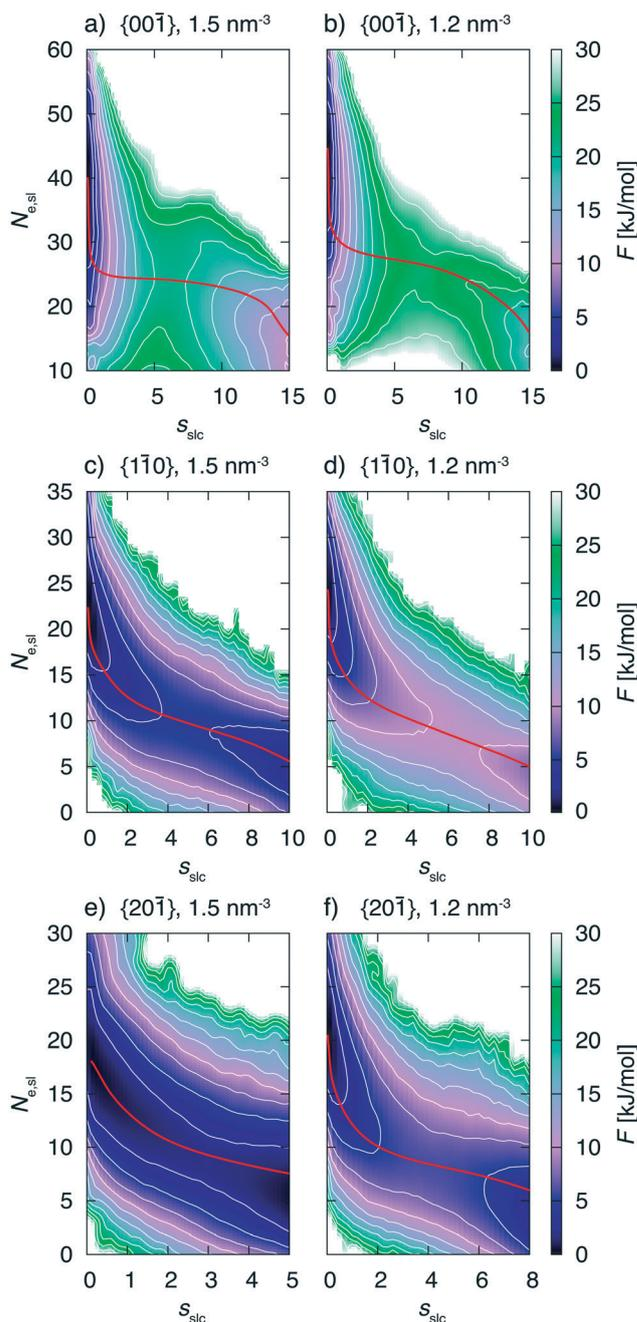
**Fig. 8** Free energy surfaces,  $F$ , in dependence of  $s_{\text{slic}}$ , the approximate number of crystalline naphthalene molecules in the surface layer, and  $N_{\text{e,sl}}$ , the number of ethanol molecules in the surface layer. The white isocontours are drawn in  $2.5 \text{ kJ mol}^{-1}$  energy steps. The red lines correspond to the minimum free energy paths. Fig. 8a)–f) show the free energy surfaces for different faces and supersaturations.
