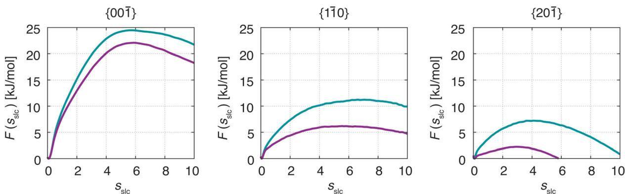
Fig. 6 Free energy,  $F(s_{\text{slc}})$ , in dependence of crystallinity of the crystal surface,  $s_{\text{slc}}$ . Green denotes the concentration at  $C = 1.2 \text{ nm}^{-3}$ , and purple denotes the concentration at  $C = 1.5 \text{ nm}^{-3}$ .
