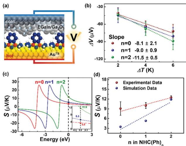
Fig. 3 (a) A schematic describing the structure of the large-area thermoelectric junction. (b) Plots of  $\Delta V$  as a function of  $\Delta T$ . (c) Simulations of  $S$  values based on the transmission function and Landauer formula (eqn (S2) and (S3) in the ESI†). The inset shows the magnification of Seebeck coefficient near the Fermi level of EGaIn. (d) Plots of experimental and theoretical  $S$  values as a function of the molecular length.
