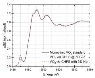
Fig. 6 V K-edge XANES of the VO<sub>2</sub> and Nb-VO<sub>2</sub> samples synthesised by CHFS. A spectrum of a commercial monoclinic VO<sub>2</sub> standard has been included for reference.
