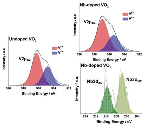
Fig. 5 X-ray photoelectron spectra (XPS) of the V 2p<sub>3/2</sub> and Nb 3d<sub>5/2</sub> environments in the (a) undoped VO<sub>2</sub> and (b) Nb-VO<sub>2</sub> samples.
