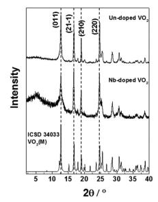
Fig. 2 XRD patterns of the VO<sub>2</sub>(M) and Nb-VO<sub>2</sub>(M) nanoparticles synthesised by CHFS. The standard XRD pattern of monoclinic VO<sub>2</sub> (ICSD 34033) has been included for reference
