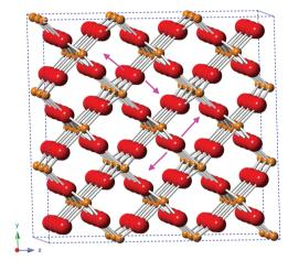
Fig. 8 Structure of monoclinic VO<sub>2</sub>, based on ICSD 34033, indicating the direction of the proposed out-of-plane oxygen displacement (purple arrows). O<sup>2-</sup>: red; V<sup>4+</sup>: orange
