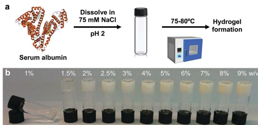
Fig. 1 Gelation of BSA solutions. (a) Protocol for hydrogel formation. (b) Image of the BSA hydrogels at different weight fractions  $\geq 1.5$  wt% BSA, together with a solution of 1 wt% BSA that did not gel after heating.
