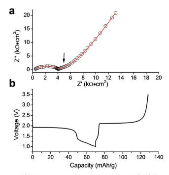
Fig. 9 (a) The impedance spectrum collected from the Li/LZP/LTP cell (LZP pellet thickness  $\sim$ 0.9 mm) at 50 °C; the arrow indicates an intermediate-frequency semicircle assigned to the LTP/LZP interfacial resistance. (b) Discharge/charge profile of the Li/LZP/LTP cell at 50 °C and 6  $\mu$ A cm<sup>-2</sup>.
