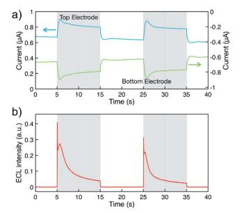
Fig. 4 (a) Measured chronoamperometric currents at the top (blue) and bottom (green) electrodes, and (b) corresponding ECL intensity. The top electrode was maintained at 2.3 V while the bottom electrode was pulsed between 0 V and -1.5 V vs. Ag, highlighted in white (redox cycling mode) and grey (annihilation ECL mode), respectively. Solution consisted of 10 mM Ru(bpy)<sub>3</sub>(PF<sub>6</sub>)<sub>2</sub> and 0.1 M TBAPF<sub>6</sub> in acetonitrile.
