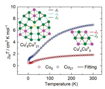
Fig. 5 The temperature dependence of  $\chi_{\rm M}T$  for  ${\rm Cu_9}$  (red circles) and Cu<sub>27</sub> (blue circles), measured in a field of 1.0 kOe. The solid black lines are the best fits (see text)
