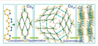
Fig. 1 The three-step tandem hierarchy in obtaining  $Cu_{27}$  from Cu (green), 5,5'-pyridyl-3,3'-bi-1*H*-pyrazole (rust and blue) and sulphate (red and yellow) and cyanide (cyan) bridges *via*  $Cu_9$ .
