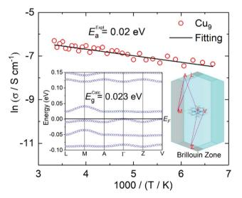
Fig. 4 Arrhenius plot of In(resistance) versus scaled inverse temperature (red circles represent experimental data and the black line is the linear fit). Inset: calculated band structure and Brillouin zone.
