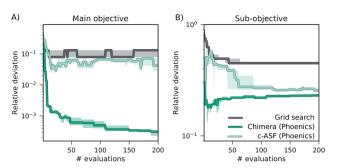
Fig. 4 Optimization traces representing the smallest relative deviations between sampled objectives and Pareto optimal objectives averaged over 25 individual optimization runs on the ZDT 2 benchmark set. Panel (A) shows deviations in the main objective, and panel (B) displays deviations in the sub-objective.
