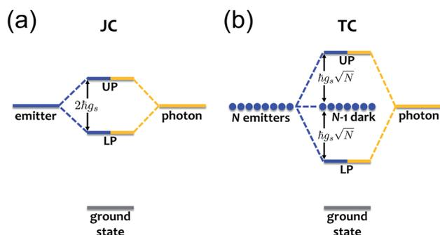
Fig. 2 (a) Jaynes–Cummings (JC) model: emitter and photon strongly couple to form hybridized states termed lower and upper polaritons (LP and UP, respectively) separated in energy by  $2\hbar g_s$ . (b) Tavis–Cummings (TC) model:  $N$  emitters interact strongly with a photon to yield polariton (LP, UP) and  $N - 1$  dark states. The latter do not couple to light and thus maintain the original emitter energy.
