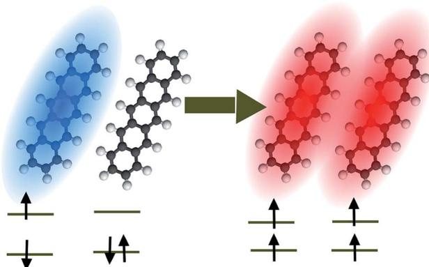
Fig. 6 Pictorial representation of singlet fission in pentacene. Blue (red) denotes a singlet (triplet) exciton.
