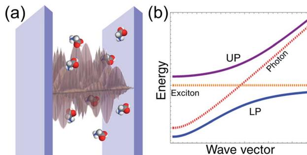
Fig. 3 (a) Pictorial representation of a set of molecular emitters embedded in a resonant planar microcavity. (b) Cavity, emitter and polariton dispersions [energy in terms of wave vector ( $\mathbf{q}$ )] according to the multimode generalization of the TC model.
