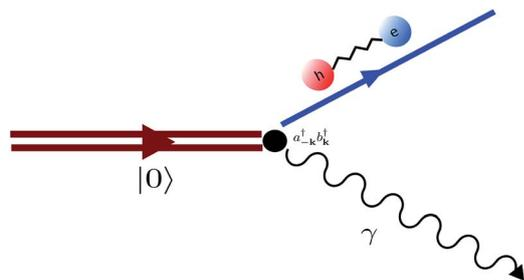
Fig. 11 Diagram representing spontaneous production of correlated exciton–photon pairs from the bare system ground-state  $|0\rangle$ . This process is significant in the ultrastrong coupling regime where light-matter couplings of the form  $(a_{-k}^{\dagger} b_k^{\dagger} + \text{h.c.})$  become relevant (see eqn (15)).
