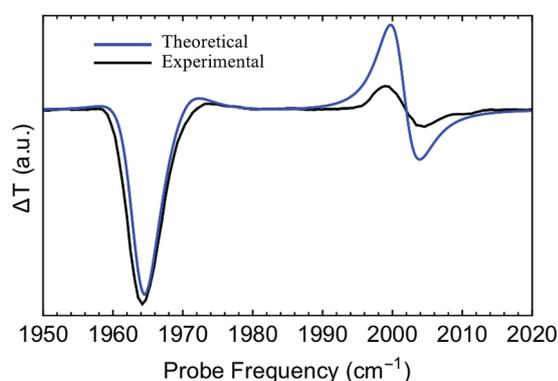
Fig. 9 Experimental and theoretical pump-probe (differential) transmission spectra of strongly coupled  $W(CO)_6$  in an optical microcavity.<sup>57</sup> These results correspond to the case where the cavity photon and the molecular vibration (asymmetric C=O stretch) are resonant.
