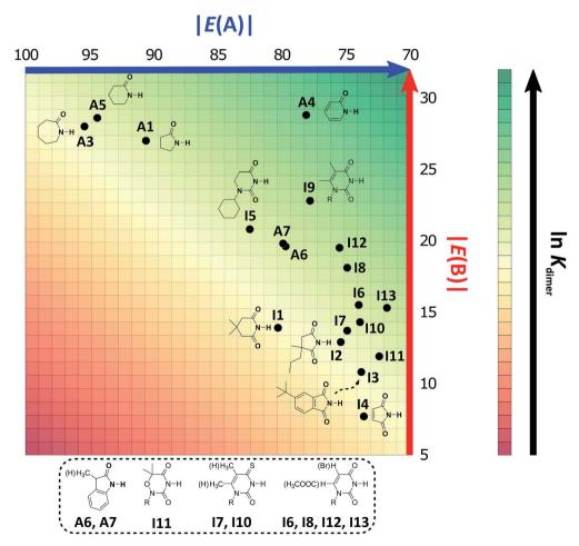
Fig. 7 2D graphical representation of the association strength of the investigated set of compounds in CDCl<sub>3</sub> as a function of acidity and basicity of the N-H and C=O groups respectively. The |E(A)| and |E(B)| values are displayed in kcal mol<sup>-1</sup>. We indicate the structure and location of each species in the acid/base plane.
