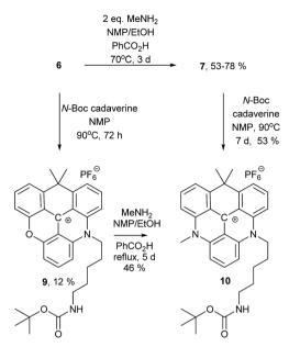
Scheme 2 Synthesis of an asymmetric substituted CDATA<sup>+</sup> dye.
