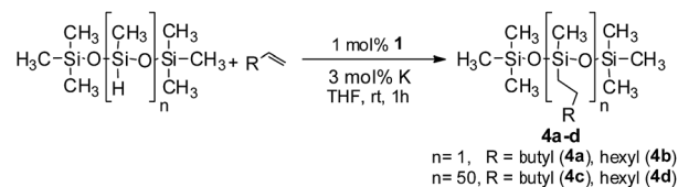
Scheme 3 The hydrosilylation of olefins by siloxanes.
