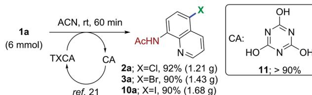
Scheme 2 Gram-scale synthesis of halogenated quinolines.
