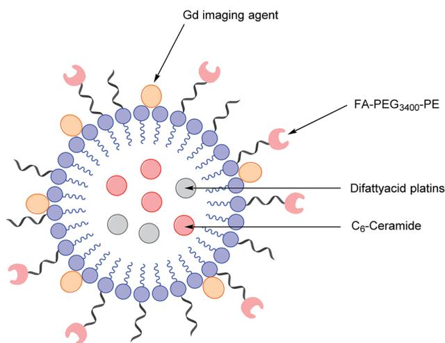
Fig. 12 Schematic representation of a NMI-350 nanoemulsion. Difattyacid platins and C<sub>6</sub>-ceramide are encapsulated in the lipid core and lipidated gadolinium and folate are attached to the surface.<sup>21</sup>
