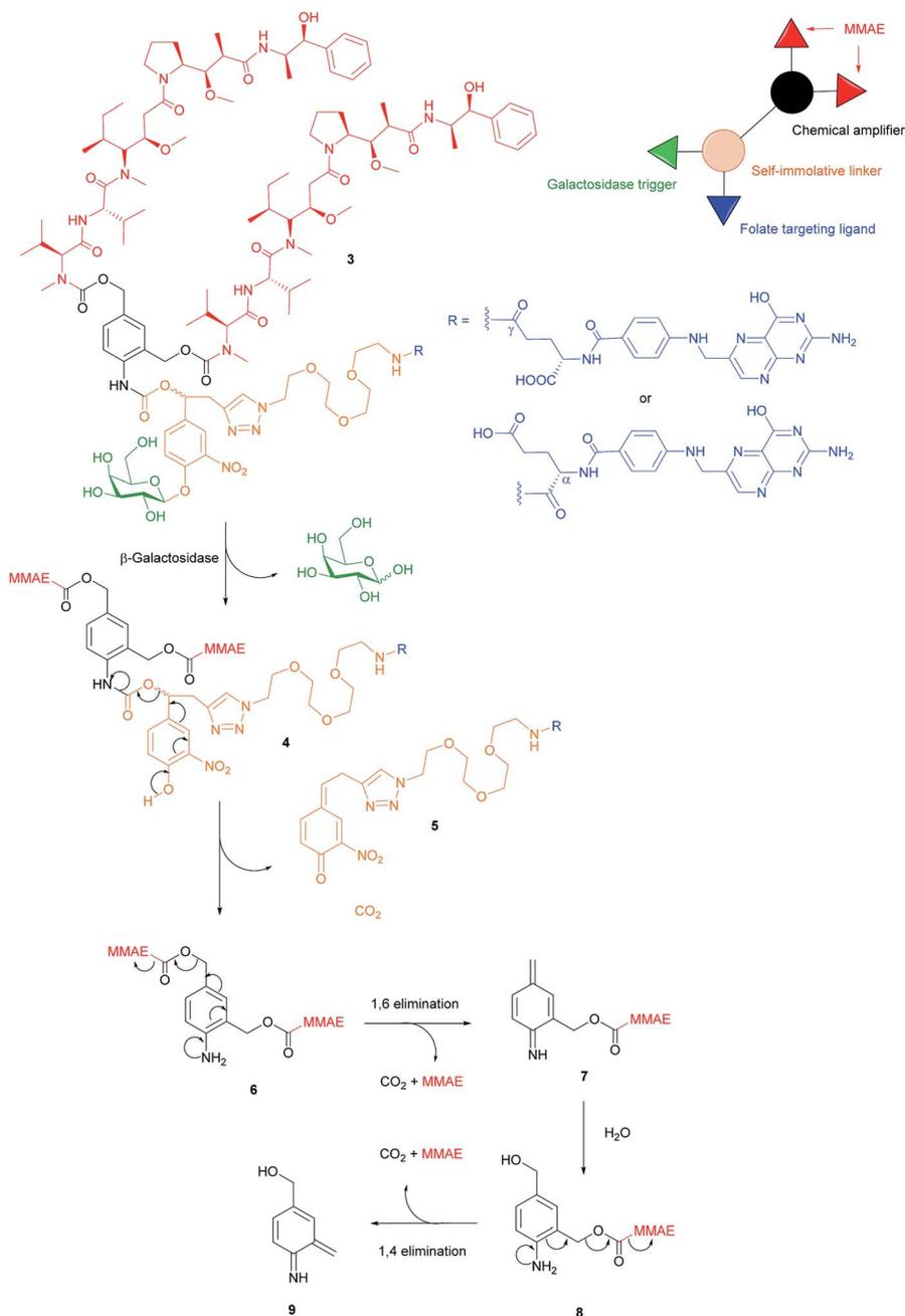
Fig. 7 Enzyme-catalysed double drug release mechanism of  $\beta$ -galactosidase-responsive folate-MMAE conjugate **3**.<sup>42</sup>
