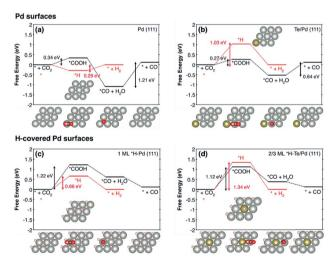
Fig. 4 The free energy diagrams of  $CO_2$  reduction to CO (black) and the  $H_2$  evolution reaction (red) for (a) Pd (111), (b) Te/Pd (111), (c) 1 ML \*H-Pd (111), and (d) 2/3 ML \*H-Te/Pd (111). Top views of the first layer of optimized geometries are shown. The light grey, dark grey, gold, red, and white balls indicate Pd, C, Te, O, and H, respectively. We note that \* represents a surface site for adsorption.
