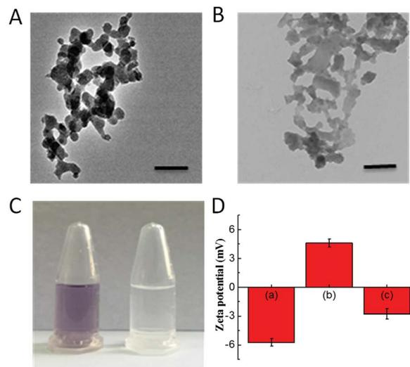
Fig. 1 Characterization of the nanomaterials. TEM of CoOOH (A) and nanophotosensitizer (B). Scale bars are 200 nm. (C) The verification of amination of CoOOH–NH<sub>2</sub> with ninhydrin experiment. On the left is CoOOH–NH<sub>2</sub>, and on the right is supernatant. (D) Zeta potential of each step of the modification: (a) CoOOH; (b) CoOOH–NH<sub>2</sub>; (c) nanophotosensitizer.
