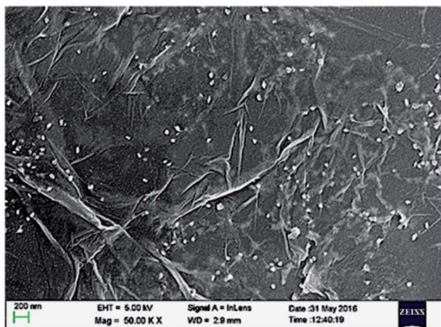
**Fig. 4** Representative FESEM micrograph of UCN@SiO<sub>2</sub>-GO nanocomposite.
