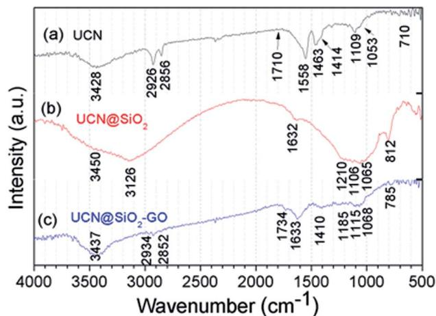
Fig. 6 FTIR spectra of (a) UCNP, (b) UCN@SiO<sub>2</sub> NPs and (c) UCN@SiO<sub>2</sub>-GO nanocomposite.
