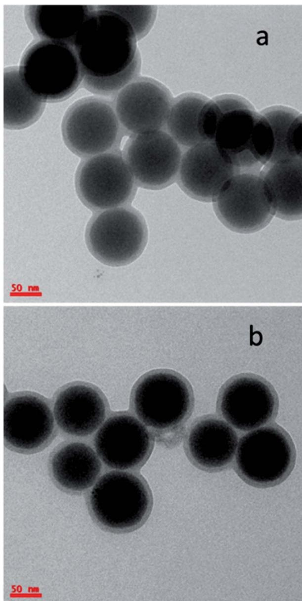
Fig. 2 TEM micrographs of (a) core shell UCN@SiO<sub>2</sub> NPs (b) at different region.
