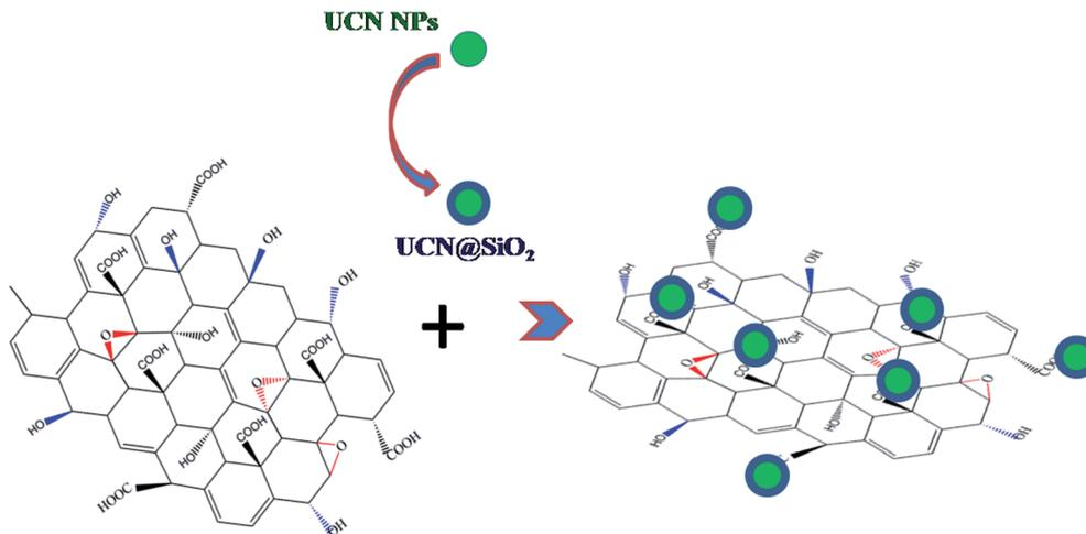
**Scheme 1** Schematic showing the concept of making UCN@SiO<sub>2</sub>-GO conjugated nanocomposite. UCN@SiO<sub>2</sub> NPs are conjugated with GO.
