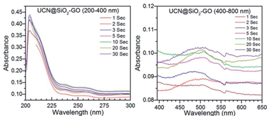
Fig. 10 Time dependent release of DOX studied through UV-Visible absorption spectra for UCN@SiO<sub>2</sub>-GO nanocomposite.
