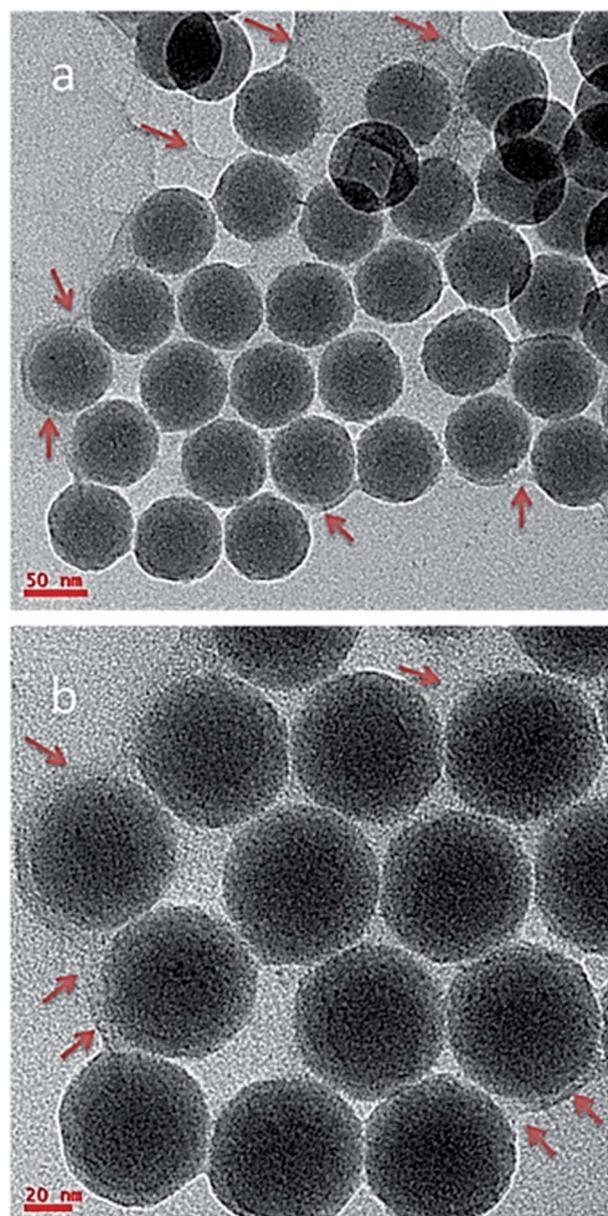
Fig. 3 TEM micrographs of UCN@SiO<sub>2</sub>-GO nanocomposite, region (a) at low magnification (b) at high magnification.
