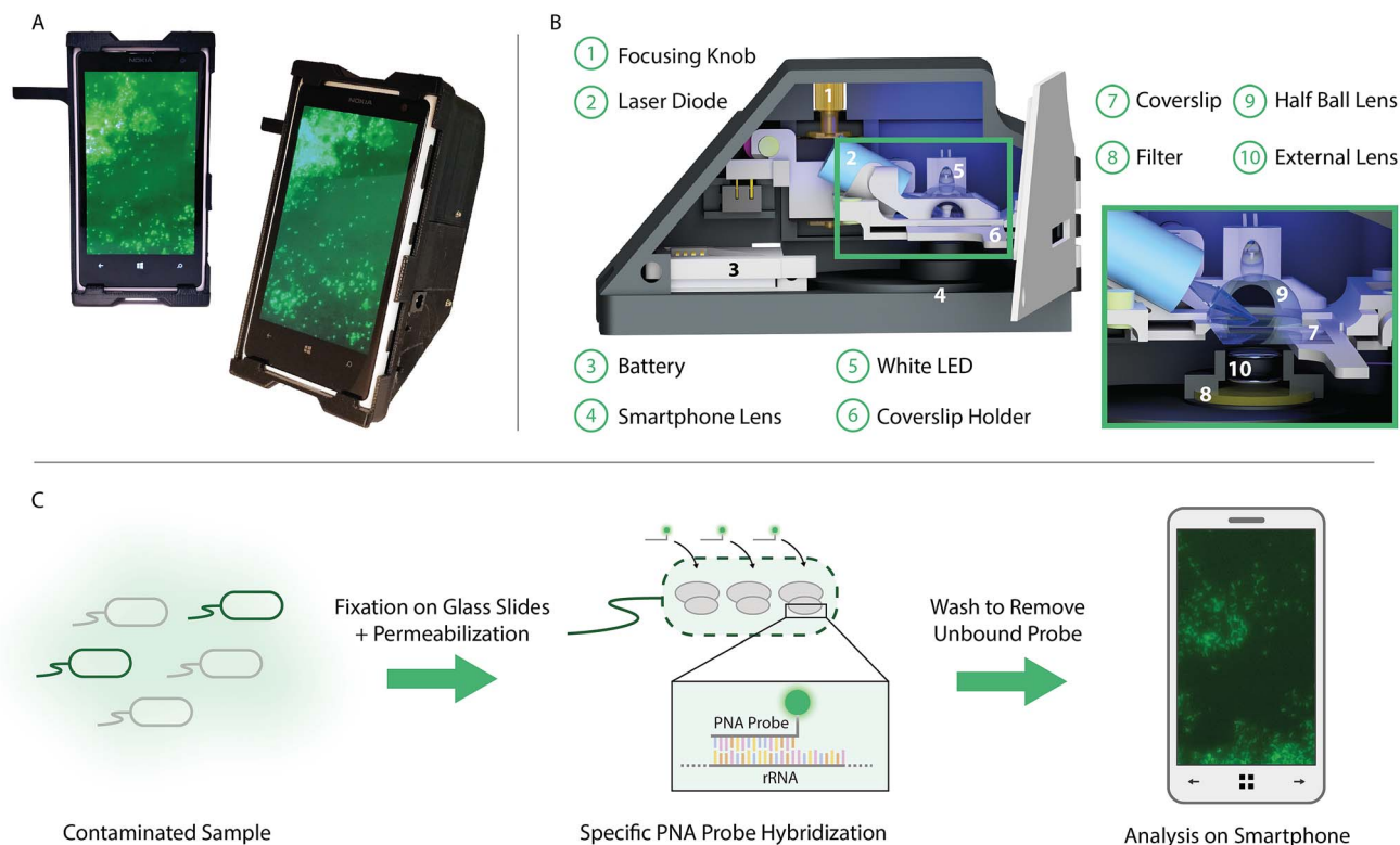
Fig. 1 Selective targeting and imaging of single bacteria on a smartphone. (A) Photographs of a smartphone microscope displaying images of fluorescently labeled Cronobacter spp. bacteria. (B) 3D illustration of the same optomechanical unit that is mounted on the smartphone in (A). (C) Schematic illustration of the bacterial detection procedure. Bacteria from the contaminated sample are fixed on 22 \times 50 \text{ mm}^2 glass slides and the bacterial membrane is permeabilized in order for the PNA probe to enter the bacteria. An Alexa Fluor 488 dye is chemically linked to the PNA probe which in turn is designed to bind specifically to certain regions of the ribosomal RNA (rRNA) of the bacteria. After washing away unbound probes, only the targeted bacteria remain fluorescent and can be imaged using the smartphone-based microscope shown in (A).
