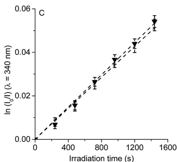
Fig. 7 First-order plots for the photooxidation of Trp (20  $\mu$ M) photosensitized by (A) TCP (■) and TCP in presence of D-mannitol (□), (B) TCP-C<sub>60</sub> (▲) and TCP-C<sub>60</sub> in presence of D-mannitol (△) and (C) TCP-C<sub>60</sub><sup>4+</sup> (▼) and TCP-C<sub>60</sub><sup>4+</sup> in presence of D-mannitol (▽) in DMF/5% water;  $\lambda_{irr} = 562$  nm.
