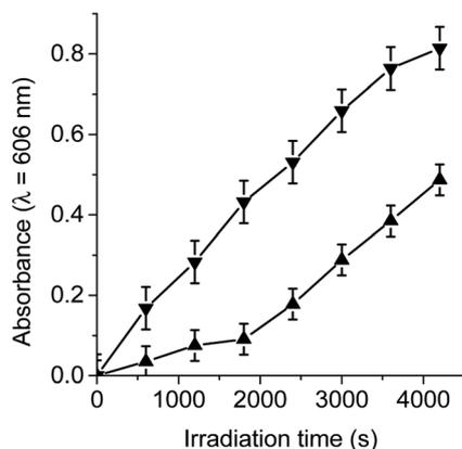
Fig. 2 Time course of  $\text{MV}^{2+}$  (0.8 mM) reduction as an increase in the absorption at  $\lambda = 606$  nm sensitized by  $\text{TCP-C}_{60}$  (▲) (3.0  $\mu\text{M}$ ) and  $\text{TCP-C}_{60}^{4+}$  (▼) (3.0  $\mu\text{M}$ ) containing TMN (0.4 mM) after 10 min irradiation periods with light at  $\lambda_{\text{irr}} = 433$  nm under an argon atmosphere in DMF/5% water.
