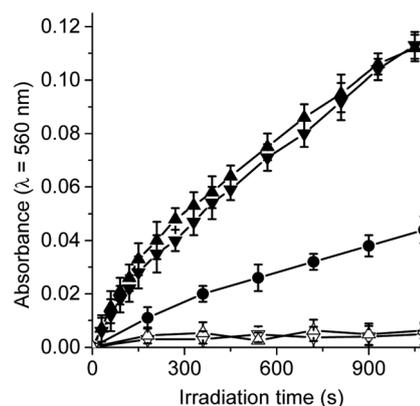
Fig. 3 Time course of NBT reduction as an increase in the absorption at  $\lambda = 560$  nm in DMF/10% water. Samples contain NBT (0.2 mM), NADH (0.5 mM) and  $\text{TCP-C}_{60}$  (▲) (1.2  $\mu\text{M}$ ) or  $\text{TCP-C}_{60}^{4+}$  (▼) (1.2  $\mu\text{M}$ ) in DMF/10% water irradiated with light at  $\lambda_{\text{irr}} = 428$  nm. Controls: NBT and NADH (●),  $\text{TCP-C}_{60}$  and NBT (Δ);  $\text{TCP-C}_{60}^{4+}$  and NBT (▽).
