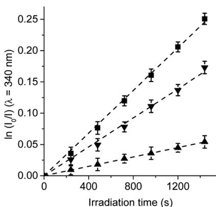
Fig. 4 First-order plots for the photooxidation of Trp (20  $\mu\text{M}$ ) photosensitized by TCP (■), TCP-C<sub>60</sub> (▲) and TCP-C<sub>60</sub><sup>4+</sup> (▼) in DMF;  $\lambda_{\text{irr}} = 428 \text{ nm}$ .
