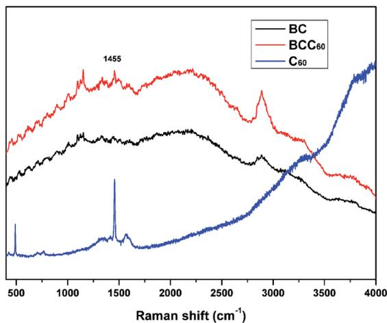
Fig. 2 Raman spectra of the BC, C<sub>60</sub> and BCC<sub>60</sub> composites.
