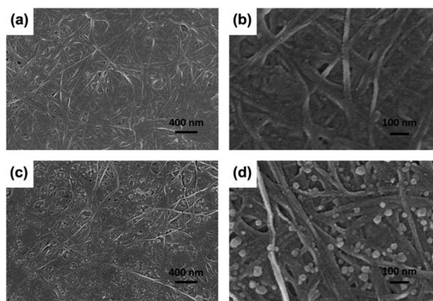
Fig. 3 SEM images of the BC and BCC<sub>60</sub> composites (a) BC, X 30k; (b) BC, X 100k; (c) BCC<sub>60</sub>, X 30k; (d) BCC<sub>60</sub>, X 100k.
