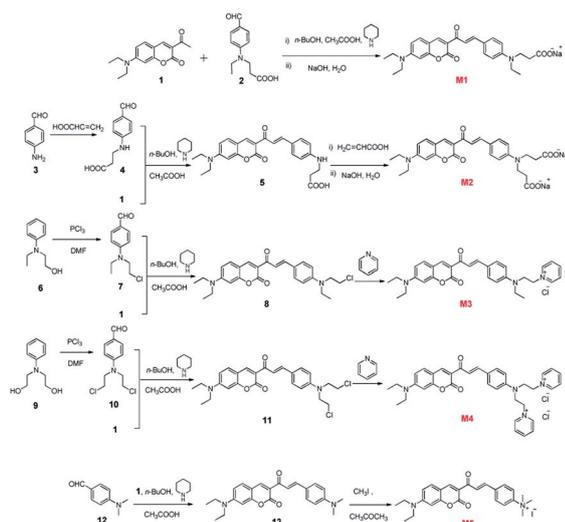
Fig. 1 Synthetic routes to targeted PSs **M1–M5**.
