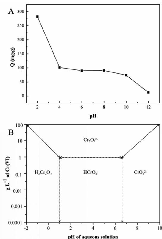
Fig. 5 (A) Effect of pH on the adsorption of Cr(vi) by GMFP: temperature, 298.15 K; adsorption time, 6 h; and initial Cr(vi) concentration, 300 mg L<sup>-1</sup>, (B) relative distribution of Cr(vi) species in water as a function of pH and Cr(vi) concentration (adapted from ref. 1).
