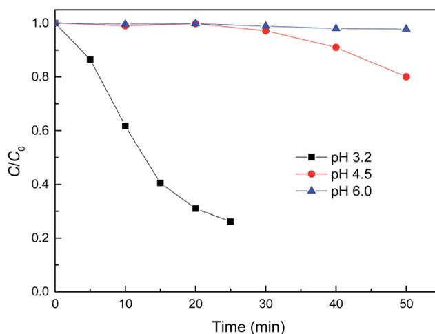
Fig. 5 Effect of initial pH on MB degradation by reduced  $\text{CuFe}_2\text{O}_4$ . Conditions:  $[\text{H}_2\text{O}_2] = 0.5 \text{ mM}$ ,  $[\text{reduced CuFe}_2\text{O}_4] = 0.1 \text{ g L}^{-1}$ ,  $[\text{MB}] = 50 \text{ mg L}^{-1}$ .
