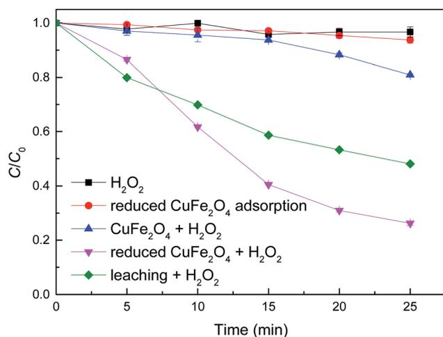
Fig. 4 Comparison of the removal efficiency of MB with different catalytic systems. Conditions:  $[\text{H}_2\text{O}_2] = 0.5 \text{ mM}$ , catalyst dosage =  $0.1 \text{ g L}^{-1}$ ,  $[\text{MB}] = 50 \text{ mg L}^{-1}$ , initial  $\text{pH} = 3.2 \pm 0.1$ .
