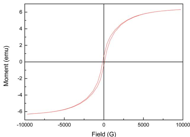
Fig. 9 Magnetization curve of reduced  $\text{CuFe}_2\text{O}_4$ .
