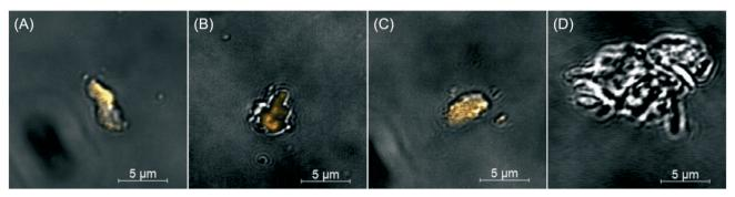
Fig. 6 CLSM images of fragments released from CdSe/ZnS-PMMA (A-C) and PMMA (D) after one day of UVC irradiation, where orange indicates any emission detected above 505 nm.
