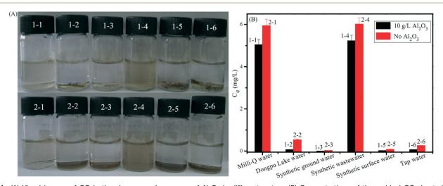
Fig. 21 (A) Visual images of GO in the absence and presence of  $Al_2O_3$  in different waters. (B) Concentrations of the residual GO sheets in the supernatant as a function of cation types and concentrations in the absence and presence of  $Al_2O_3$  in natural and synthetic waters.  $C_{(GO)initial} = 6$  mg  $L^{-1}$ , m/V = 10 g  $L^{-1}$  (i.e.,  $Al_2O_3$  concentration). <sup>84</sup> Reprinted with permission from ref. 84. Copyright 2014, American Chemical Society.
