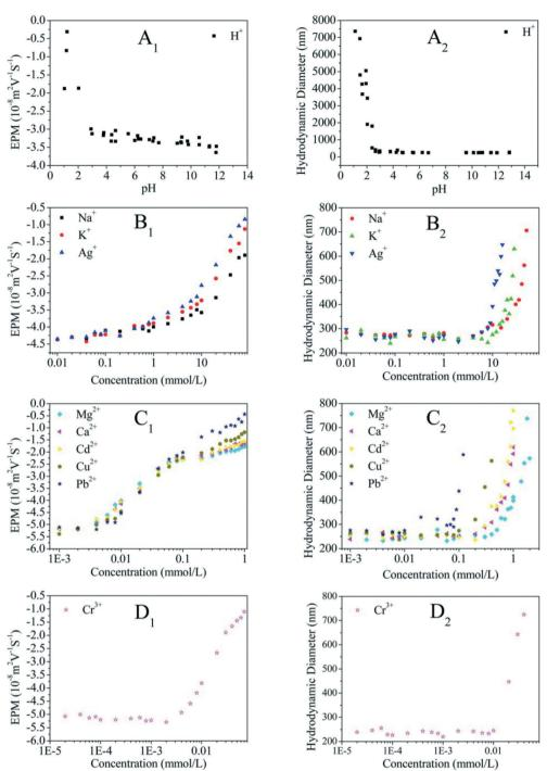
Fig. 7 Electrophoretic mobility (EPM) and hydrodynamic diameter of GO as a function of the cation concentration of H<sup>+</sup> (A<sub>1</sub> and A<sub>2</sub>), monovalent metal cations (B<sub>1</sub> and B<sub>2</sub>), divalent metal cations (C<sub>1</sub> and C<sub>2</sub>), and trivalent metal cations (D<sub>1</sub> and D<sub>2</sub>). The Reprinted with permission from ref. 71. Copyright 2016, American Chemical Society.
